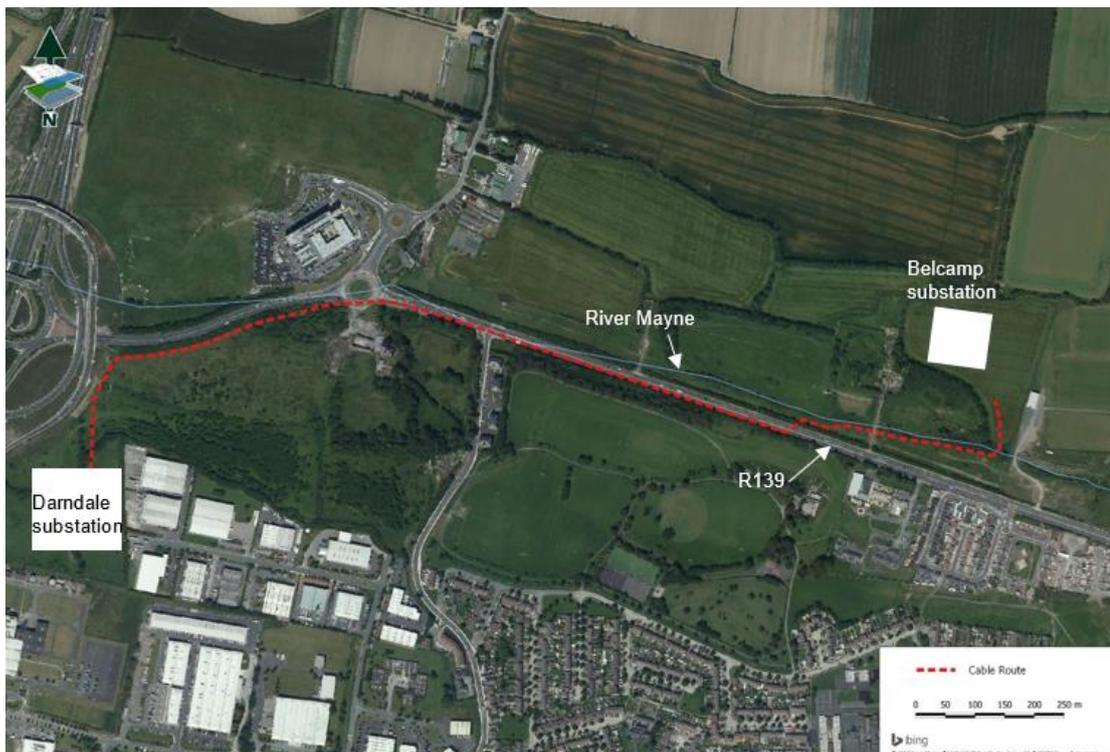
**Figure 1.1** Proposed Route of 110kV Underground cable installation
